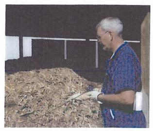
Figure 4. Checking internal temperatures with a composting thermometer is a quick way to determine if moisture and other conditions are suitable for rapid decay and pathogen reduction. (Photo by Tom Glanville, Iowa State University.)
